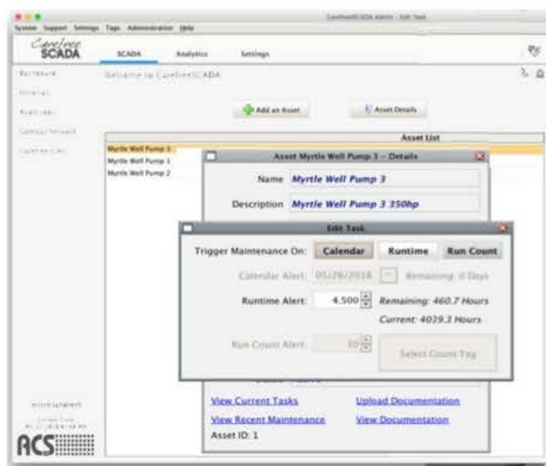
Asset preventive maintenance task configurations in AM-enabled SCADA system
